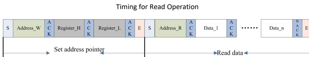
The diagram above is the timing sequence of the host reading data from GT911. First, the host issues a Start condition and sends 0XBA (address bits and R/W bit; R/W bit as 0 indicates Write operation) to the slave device.
